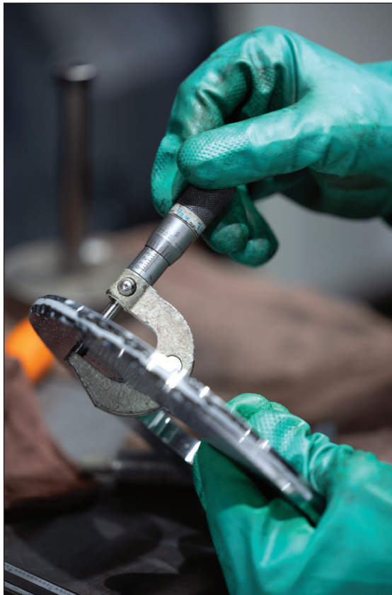
A Dubuque Stamping & Manufacturing Inc. employee uses a micrometer to measure a part.
